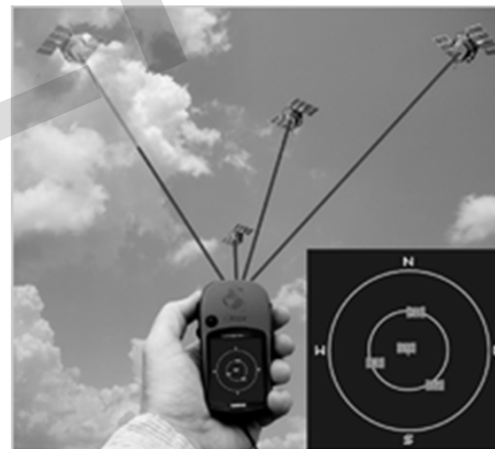
Navigation satellites with good geometry for Geometric Dilution of Precision (GDOP).
